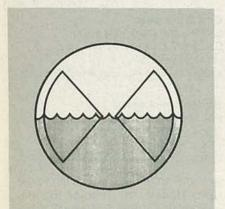
FIG. 6—CAPACITIVE LEVEL SENSOR is the one most often used today for electronic levels and inclinometers. As the device tilts, the high dielectric constant of the liquid will change the differential capacitance on the plates.
