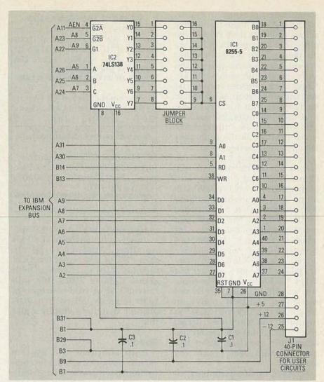
FIG. 1—ADD THREE 8-BIT PARALLEL PORTS for I/O experiments using this simple circuit. The jumper block lets you assign port addresses from 0200h to 02FFh.
