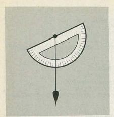
FIG. 4—THIS SIMPLE INCLINOMETER can be created by using nothing but a plumb bob and a protractor. You sight along the base of the protractor base and then read the angle.
