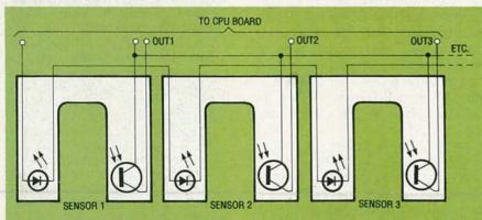
FIG. 4—SCHEMATIC DIAGRAM of the grass-sensor assembly.
