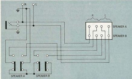
FIG. 5—THE MATRIX SURROUND CIRCUIT used in receivers such as Teac's AG-75 extracts ambience information from a pair of stereo signals by finding the difference
