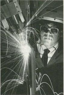
GE R&D CENTER ENGINEER ANGEL L. ORTIZ, JR puts the face-pumped laser to work drilling holes in a ½-inch thick plate of superalloy; in other tests it's managed to drill through more than two inches of superalloy. The solid-state laser's average power output of 1,000 watts from a single laser head opens the door to development of industrial laser systems that can cut and drill space-age metals and alloys with unprecedented speed and precision.
