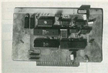
FIG. 8—FULLY ASSEMBLED CPU BOARD.
