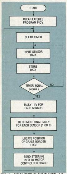
FIG. 5-SIMPLIFIED FLOW CHART of the computer program.
