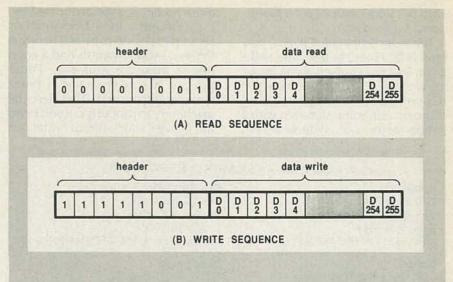
FIG. 2—THE ECONORAM GETS INTERROGATED by use of 264 sequential timing pulses. Once started, the sequence must get completed in its entirety. See the DS2222 data sheet for additional details.
