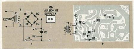
FIG. 7—A FULL-WAVE BRIDGE RECTIFIER as supply #1; (a) is the relevant segment of schematic, (b) is the relevant segment of the parts placement diagram. Remeber to reverse D1–D4 for a fixed-negative version. The connections for a full-wave bridge are shown in Fig. 7, and don't forget to add JU8. You can also make supply #2 on top any version, whether positive, negative, fixed, or adjustable.
