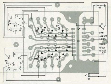
FIG. 5—PARTS-PLACEMENT DIAGRAM FOR THE ROTARY-SWITCH version of the PXO-1000 circuit.
