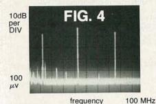
A cordless phone (base station) is probed near its 38.970 crystal in fig. 4. Both 39 MHz and its second harmonic are obvious. The lowest line at 10.245 is also obvious and can be established by probing the adjacent 10.2 crystal, which then shows 10MHz as higher level than 38MHz. We have established receiver RF oscillator/system operation in seconds with no connection, information, schematic, etc.!
