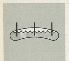
FIG. 5—AN ELECTROLYTIC LEVEL is one older electronic inclinometer. As the device tilts, the bridge resistance between the sensing pins will change. Bromine is one possible liquid.
