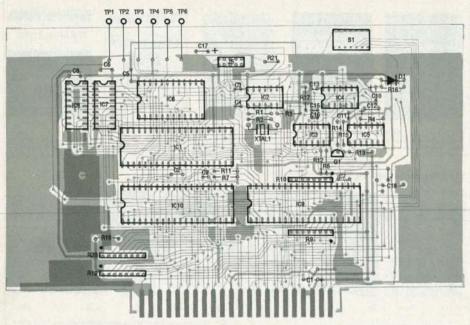
FIG. 7—ASSEMBLE THE COMPONENTS according to this parts-placement diagram.
