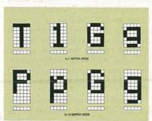
FIG. 3—HERE ARE SOME EXAMPLES of letters formed using the  $5\times7$  and  $5\times10$  dot-matrix formats.
