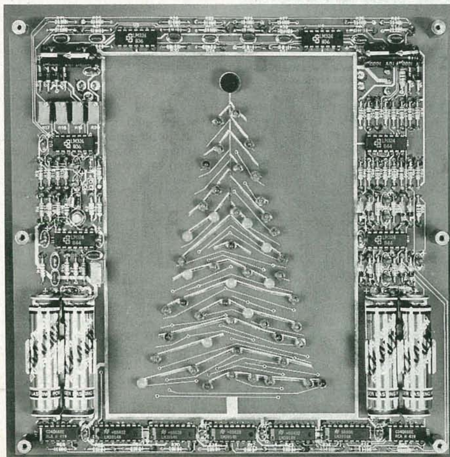
FIG. 7—THE SPACERS THAT HOLD THE BOARD in place in the metal frame should be installed early to prevent damage to soldered components.
