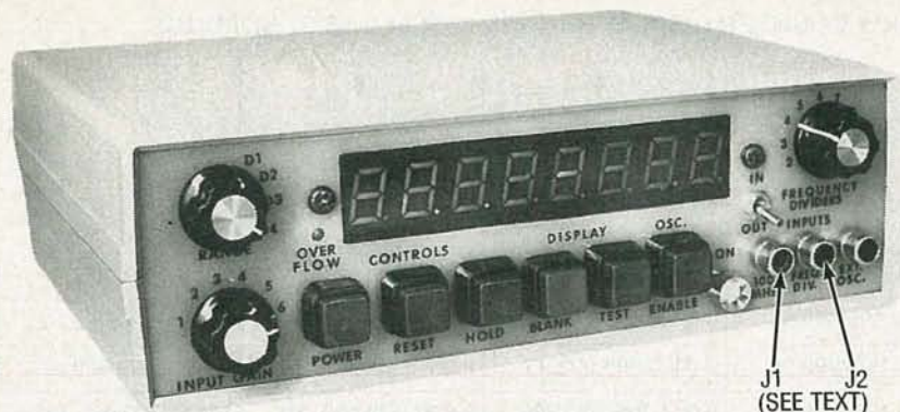
FIG. 6—THE FINISHED FREQUENCY COUNTER, shown in display-test mode, with all digits and decimal points lit. J1 and J2 are wired together, but one is unnecessary (see text).
