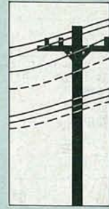
PRIMARY DISTRIBUTION LINES (4–35KV) 1–5 \mu T, WITH MAGNETIC FIELD DROP OFF AT 1/r^2
