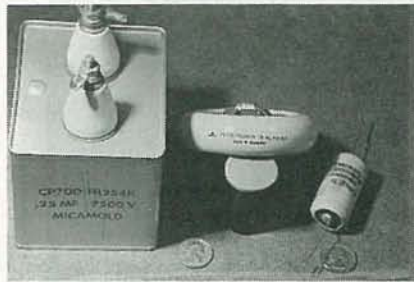
FIG. 9—HIGH-VOLTAGE CAPACITORS. A 0.25 \mu\text{F} , 7.5-kilovolt capacitor is on the left; a 100 pF, 15-kilovolt capacitor is in the middle; and 0.0005 \mu\text{F} , 5-kilovolt capacitor is on the right.
