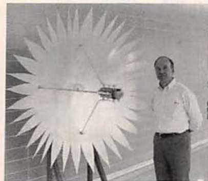
DR. EDWARD B. JOY, PROFESSOR OF ELECTRICAL ENGINEERING at Georgia Tech, shows antenna dish with flower petal edges that improve the antenna's performance.
