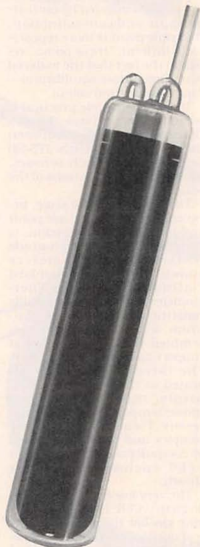
FIG. 2—FIXED POINT CELL. The graphite crucible, visible through the quartz enclosure, contains a high-purity metal. (Courtesy of YSI Inc.)
