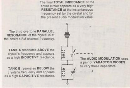
FIG. 4—SIMPLIFIED SCHEMATIC of the linear reactance modulator.
