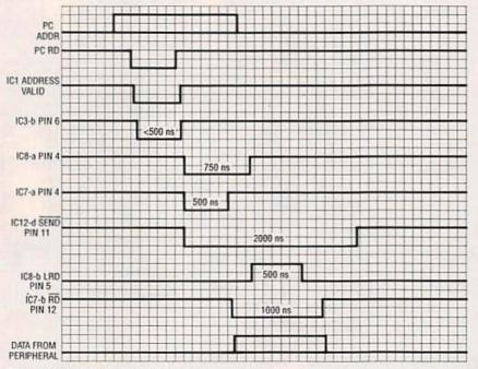
FIG. 3-11000 READ, or "in" timing sequence.
