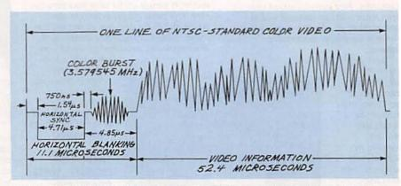
FIG. 1—A VIDEO WAVEFORM is an extremely complex signal. If you would like to know how your local cable company does their scrambling, take a few scope photos of the scrambled signal or make some sketches of it, and send them in to us.
