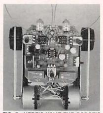
FIG. 7—HERE'S WHAT THE ROBOT'S board looks like close up. You can also see how the feelers work.
