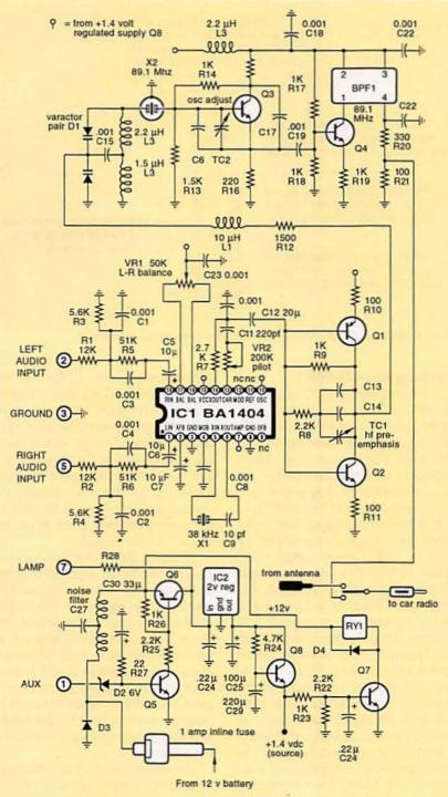
WARNING: Be sure to current limit the AUX input with an external 1K resistor!
