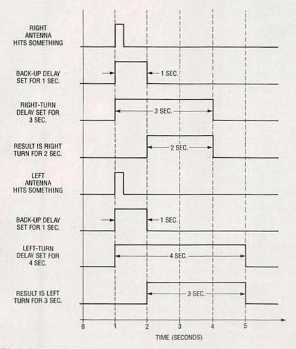
FIG. 2—TIMING DIAGRAM. Either antenna will reverse both motors and the robot backs up. When the back-up time is over, one of the motors continues in reverse, causing the robot to turn away from the object.
