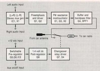
FIG. 2—MOST LOW-END FM WIRELESS BROADCASTERS simply will no longer work because nearly all the newer synthesized receivers now *demand* precisely on-channel stations. The Pioneer CD-FM-1 (block diagram shown here) generates exact-frequency stereo FM signals. The CD-FM-1 is easily made wireless.
