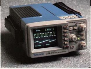
With this new 60 MHz digital oscilloscope, Tektronix takes handheld performance to an even higher plane! The 224 packs more power per pound than any other product and — with its on-board rechargeable batteries — goes wherever duty calls. With its exclusive IsolatedChannel<sup>™</sup> architecture, you can make two-
