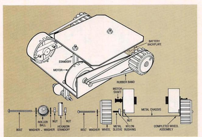
FIG. 4—FOLLOW THIS DIAGRAM as a mechanical assembly guide. Note that the motors come attached to the metal chassis plate, and can break lose if you flex or bend the chassis.
