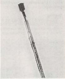
FIG. 3—THE TEMPERATURE-SENSING diode can be sealed in a length of glass tubing and sealed with RTV silicone. You must use a shielded cable between the probe and the measuring circuit.
