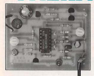
This solid-state thermostat can replace those old mechanical units—at a cost of less than twenty dollars!
