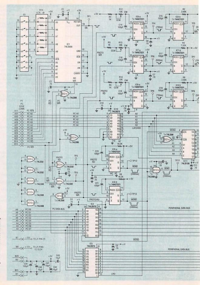
FIG. 4—11000 SCHEMATIC. The 11000 can talk to 32 locations within 256 peripheral devices to provide tremendous flexibility.
