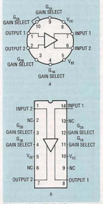
FIG. 2—TOP VIEWS OF 592 and 733 packages: (a) metal can and (b) ceramic and plastic DIP.
